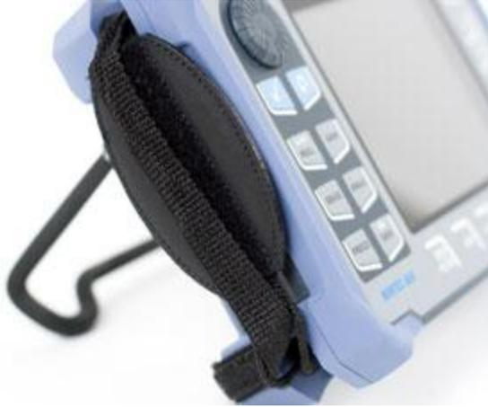
The NORTEC 600 weighs only 1.6 kg and is delivered with a factory-installed hand strap that provides direct thumb access to the key controls, offering genuine handheld versatility to operators.
